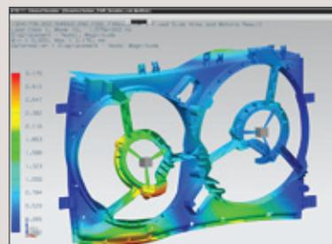
Structural and modal simulation is conducted to ensure that the mounting scheme will support the new design variant with the required performance parameters.
