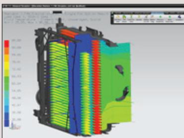
Using a combination of NX Flow and NX Thermal it is discovered that a radiator assembly isn't pulling enough heat out of the system. It is only achieving 36kW whereas 41kW is required for this engine.
