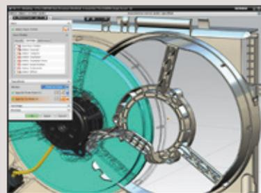
The single fan design concept is quickly modified using Synchronous Technology to take the existing design (including fan and mounting sub-assemblies) and create a two fan variant.
