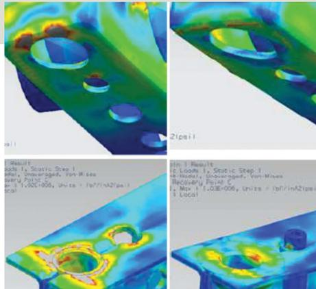
Reproduction of yielding on rear suspension parts, with solution shown in second image, using NX CAE.
