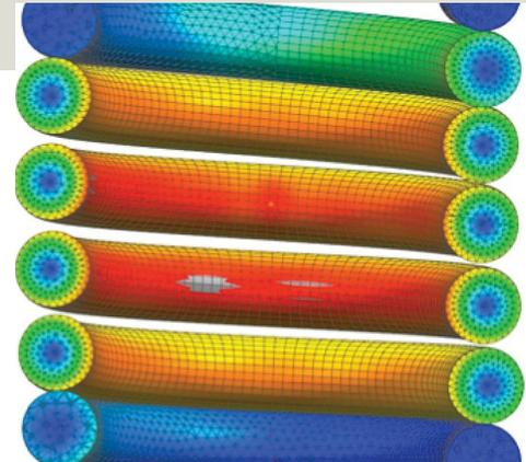
Valve spring shear stress distribution using NX CAE simulation.
