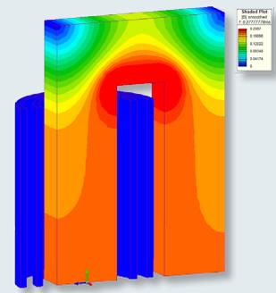
Flux-density of the single-phase transformer
