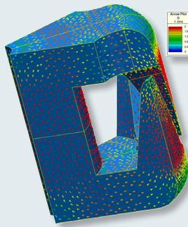
Flux-density of the Claw-pole alternator
