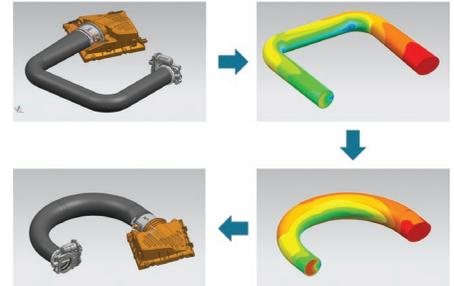
Drive design through simulation-based geometry optimization.
