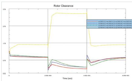
The multiphysics environment streamlines bi-directional thermal-structural coupling to study blade clearance in an aircraft engine.
