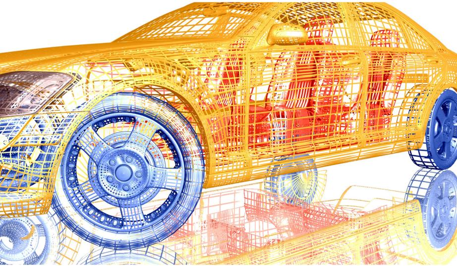
SAToolkit Pro's performance changes the game with accurate solutions of very large beam, shell and solid models over the complete frequency band. This model, consisting of 600,000 solid elements, 980,000 nodes and 250 modes, was solved in 120 minutes for all 3 axes.
