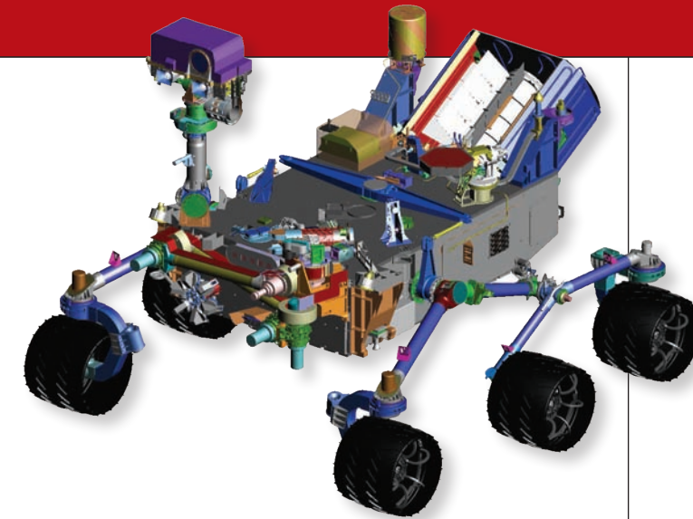
A 3D CAD rendering of the MSL rover in fully-deployed 'traverse' mode. Different systems are color coded.
