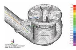
handles disjoint meshes at the fluid/solid boundaries. This unique technology of thermally coupling the disjoint solid and fluid meshes provides a complete solution for simulation of conjugate heat transfer problems.
